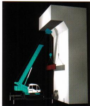
This illustration shows the limits and controls on boom height and operating radius. Limits and controls on swing angles are also possible.
